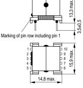
Recommended hole arrangement (view in mounting direction)
